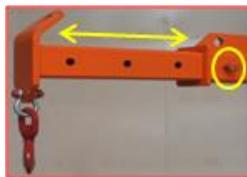
Slide the adjustable bars left and right into the sleeve of the attachment part of the implement until the correct setting is achieved in relation to the dimensions of the products or materials to be treated.
