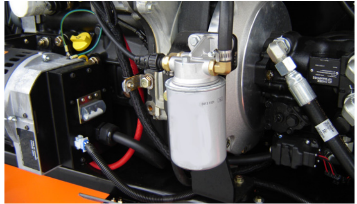
C. Brandstoffilter – Deutz TD2.9 (op motor)
