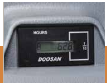
Hour meter (from ground level)
