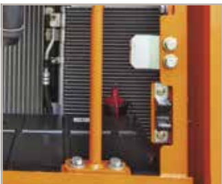
Battery cut-off switch
