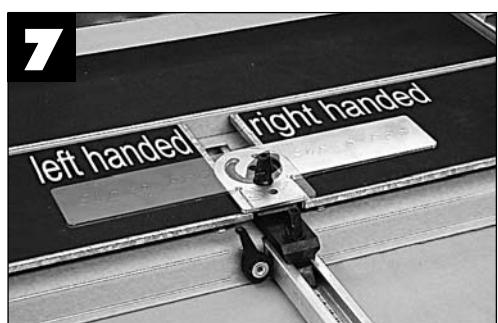
**DLA PRAWIDŁOWEGO WYREGULOWANIA UCHWYTU KĄTOWEGO NA 90°, USTAWIĆ GO POŚRODKU KRAWĘDZI TNĄCEJ STOŁU ROBOCZEGO, ZANIM ZOSTANIE PONOWNIE DOKRĘCONE POKRĘTŁO USTALAJĄCE.**
