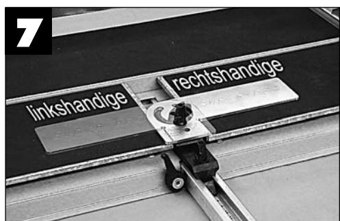
**LIJN DE HOEKHAAK UIT MET HET MIDDEN VAN DE SNIJBALK OP HET WERKBLAD, OM HEM PERFECT 90° TE ZETTEN, VOORDAT U DE VERGRENDELKNOP WEER VASTDRAAIT.**
