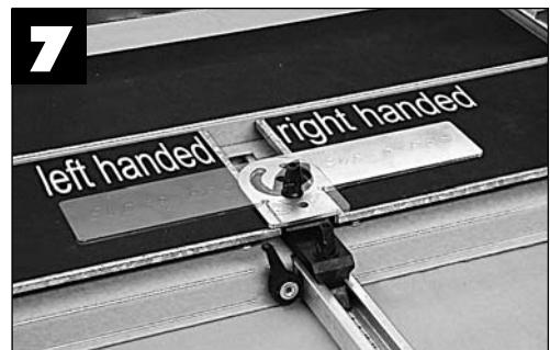
**THE BLOCKING KNOB MUST BE ALIGNED WITH THE CENTRE OF THE CUTTING SIDE OF THE WORKTOP BEFORE TIGHTENING IT, IN ORDER TO OBTAIN A CORRECT 90° POSITION OF THE FENCE.**
