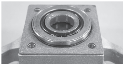
Fig. 12 - View of the Lower Driver Body Assembly when removed from the post driver.
